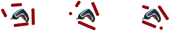
Fig. 21: Proposed partial cages using the VAE cage acquisition method. The novel object (hand drill) is feed into the cage acquisition and the best three cages from the closest object in the dataset are shown (in red).
