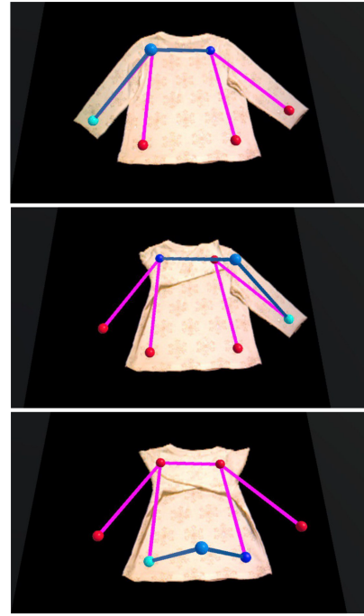
Fig. 6: Different folding actions proposed by the robot during the automatic folding execution , pick-nodes displayed in light blue, place-nodes in blue.
