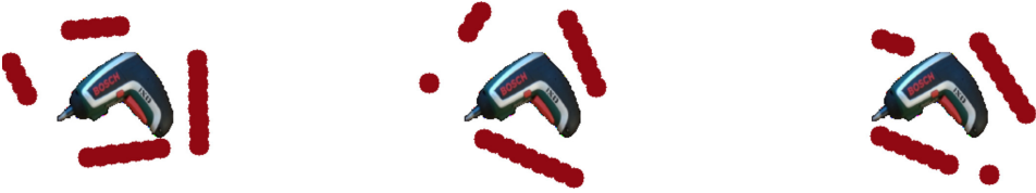
Figure A.21: Proposed partial cages using the VAE cage acquisition method. The novel object (hand drill) is feed into the cage acquisition and the best three cages from the closest object in the dataset are shown (in red).
